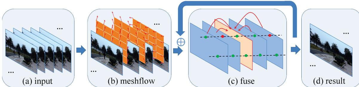
**Fig. 1.** Our system pipeline. (a) The input noisy video. (b) The meshflow is estimated between adjacent frames. (c) All the neighboring frames within a local temporal window are warped towards the central frame according to the meshflow. The denoised frame is generated by fusing of warped frames with consistent pixels identification. (d) The video is denoised frame by frame with a moving temporal window.
