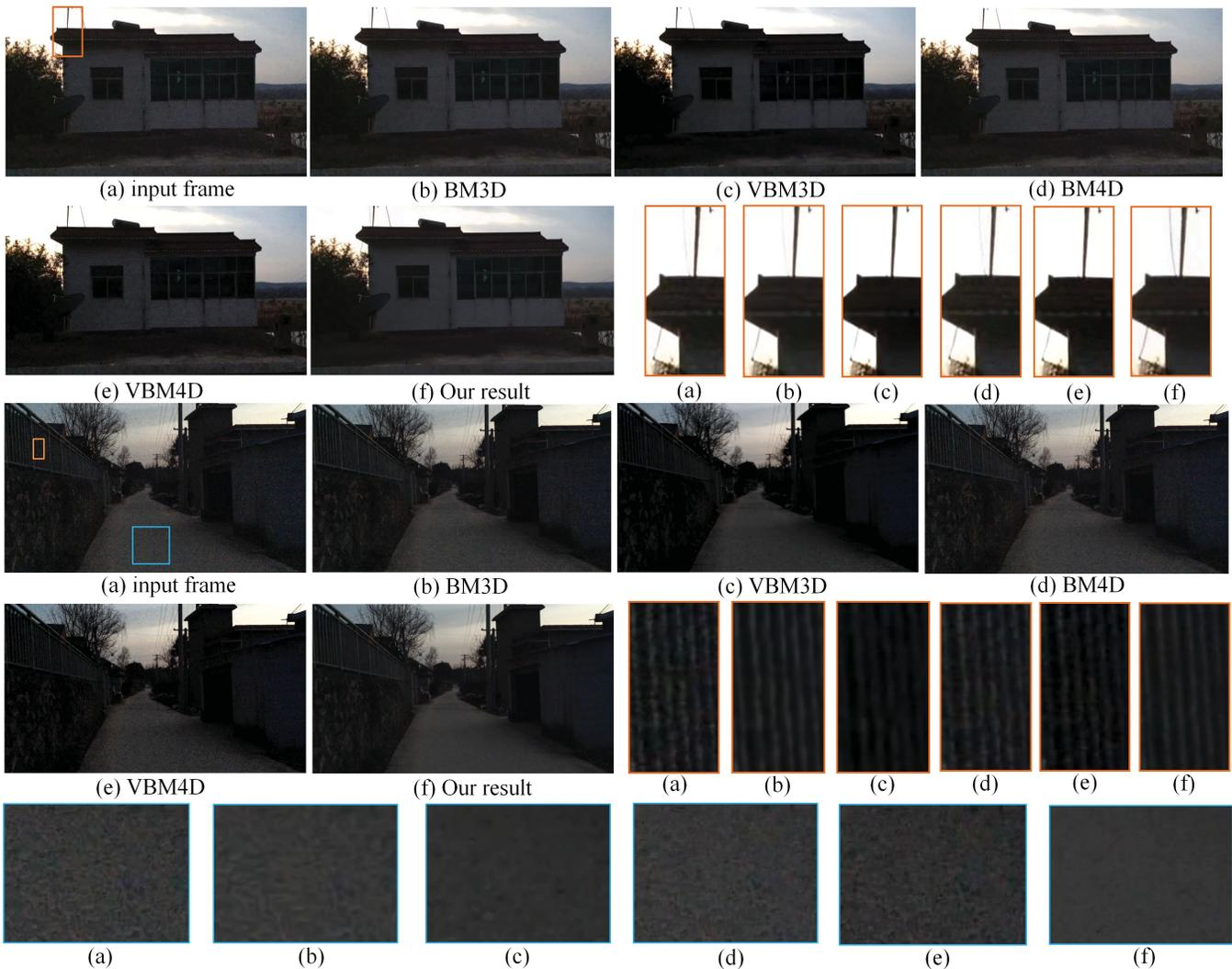
**Fig. 6.** Comparisons with various methods, including (b) BM3D [5], (c) VBM3D [19], (d) BM4D [20] and (e) VBM4D [21]. Please zoom in for clearer comparisons and refer to the video for comparisons of the temporal consistencies. Our method can keep image details as highlighted by the rectangle in the first example while suppress the noises effectively as highlighted in the second example.
